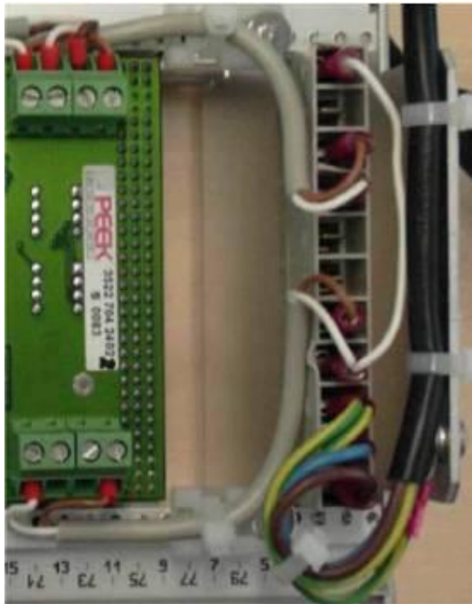
Figure 40 Connection diagram Power supply (PSU) interfaces
