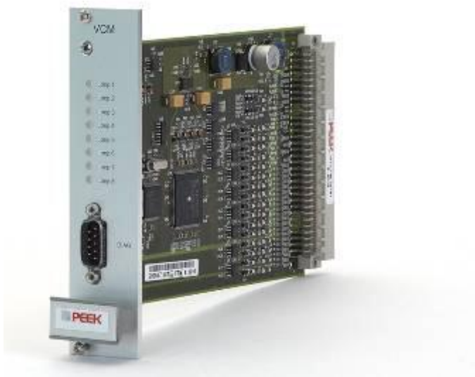
Figure 33 Layout VECOM Control Module (VCM)
