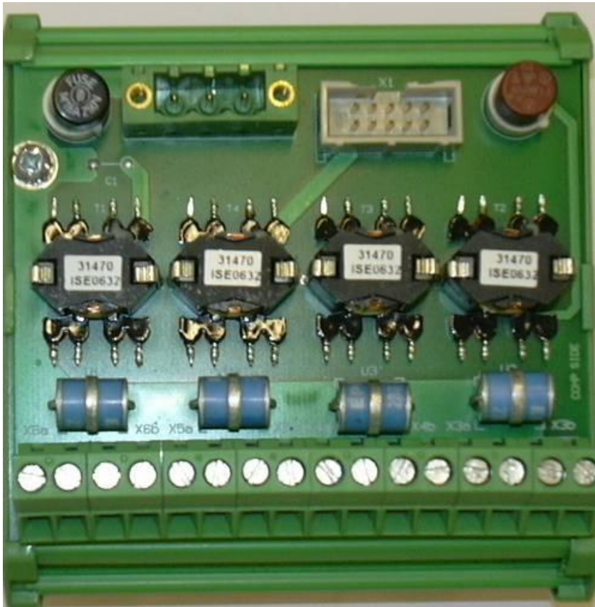
Figure 48 Loop distribution panel (LDP-T)
